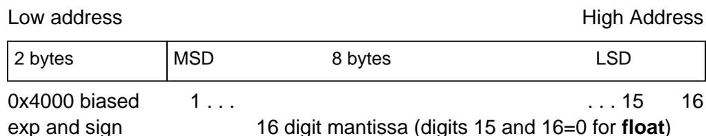
**Figure 2.2: Internal TI BCD Floating-Point Representation**
