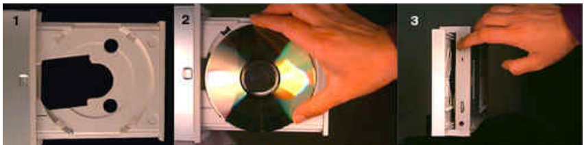
Figure 2 - Inserting DVD or CD Vertically
