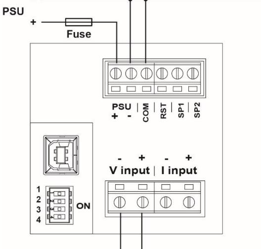
Note: When using a DC PSU, always link PSU negative to COM terminal
