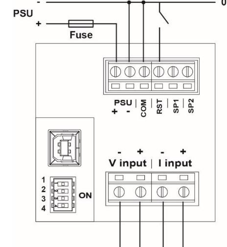
Note: When using a DC PSU, always link PSU negative to COM terminal
