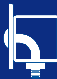
Corner bolts prevent side wall deformation
