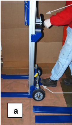
Engage the brakes by pressing down on the brake actuator
