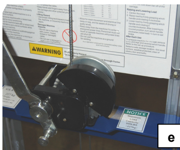
Slide the handle onto the handle connector
