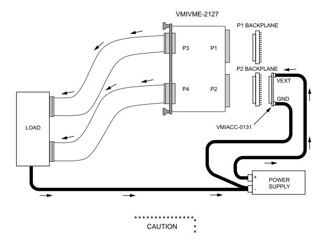
THE ARROWS DENOTE CURRENT FLOW. IT IS VERY IMPORTANT THAT THE CURRENT IS RETURNED TO THE POWER SUPPLY AS SHOWN AND IS NOT RETURNED THROUGH THE VMIVME-2127.
