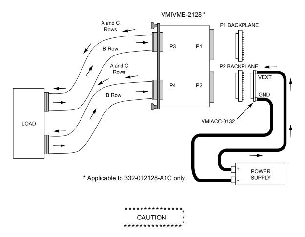
THE ARROWS DENOTE CURRENT FLOW. IT IS VERY IMPORTANT THAT THE CURRENT DOES NOT EXCEED 40 AMPS.
