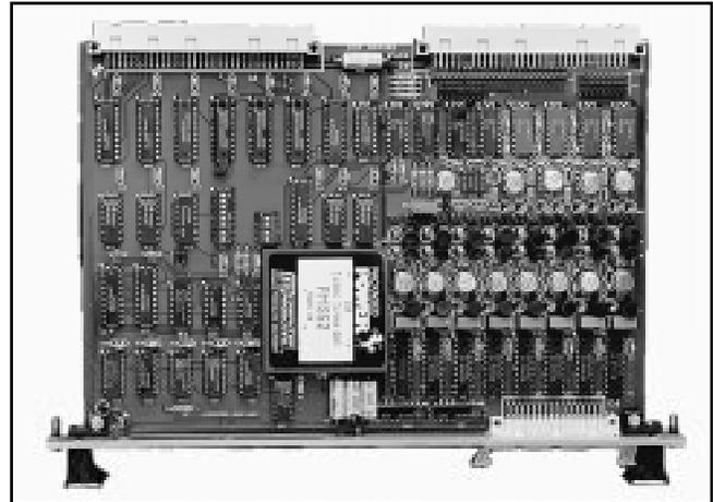
**Analog Output Testing:** Any one of the eight analog outputs may be switched to the analog output test bus (Test Bus 2). This bus is routed through the P2 AMXbus analog backplane to an Analog-to-Digital Converter (ADC) board which is used to verify each DAC channel on the VMIVME-4105 board.
