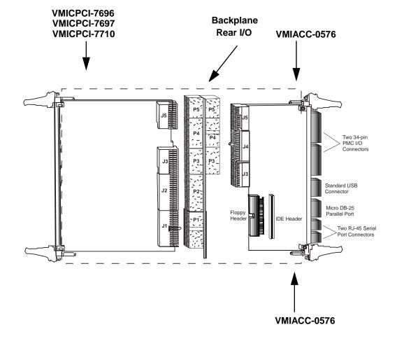
Figure 1. VMIACC-0576 and Rear I/O with VMICPCI-7696, -7697, or -7710
