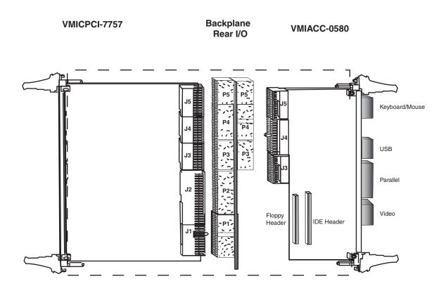
Figure 1. VMIACC-0580 and Rear I/O with VMICPCI-7757
