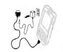
Or place the WPA206 into the Docking Station (first connect the power supply to the Docking Station).
