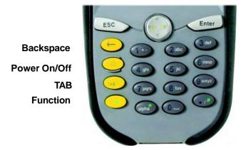
**ON/OFF** When the unit is off, pressing the On/OFF key will turn the unit on.
