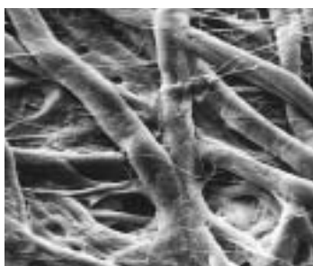
Whatman cellulose filter papers exhibit particle retention levels down to 2.5 \mu\text{m} .
