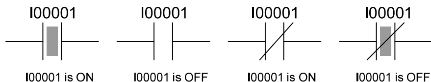
Figure B17.2 Conduction States of Contact A and Contact B
