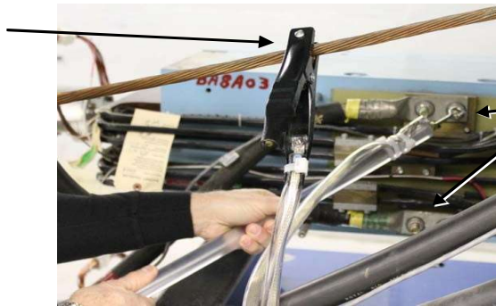
Figure 4-1: Clamp the Grounding Lead, then touch the positive and negative leads
