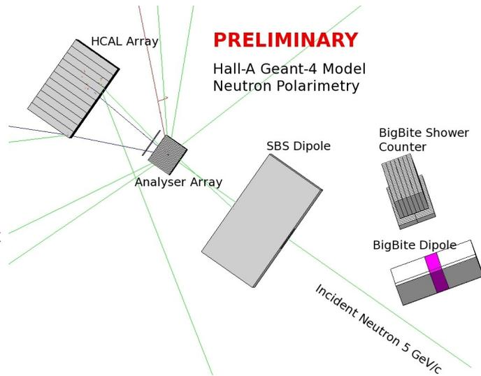
Fig. 1: Preliminary layout of the neutron polarimeter showing tracks from a single neutron interaction in the analyser array and HCAL calorimeter.
