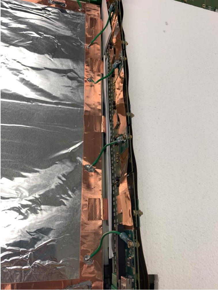
Ground between top shield and flexible backplane APV cards
