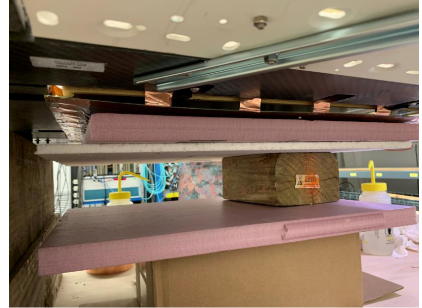
How we slowly elevate the bottom shielding. Probably want to create a more permanent apparatus if doing this shielding more.
