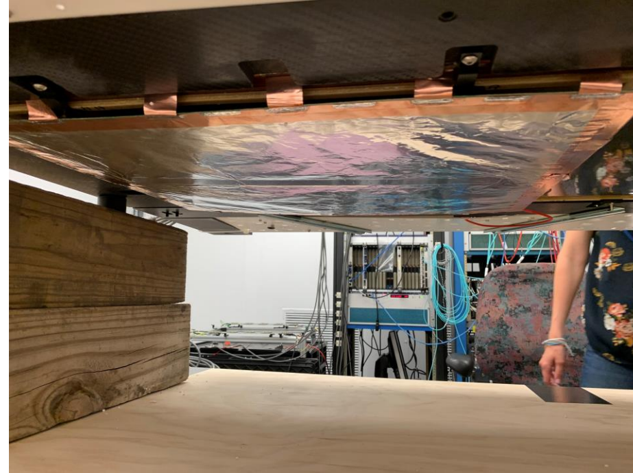
Shielding on bottom of GEM module
