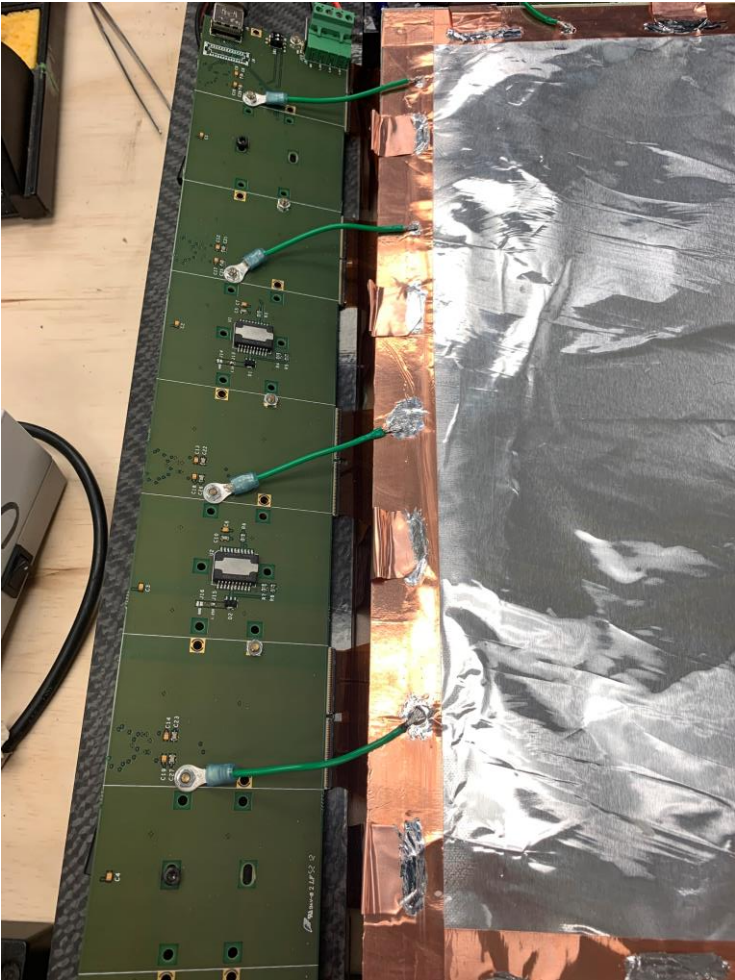
Ground between top shield and ridge backplane APV cards
