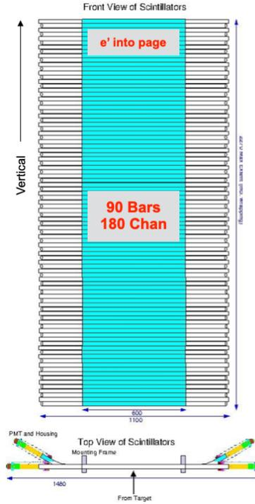
Figure 1: BigBite Timing Hodoscope components.
