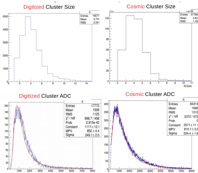
Figure 2: Cluster size and amplitude of digitized elastic electron hits and real cosmic hits.
