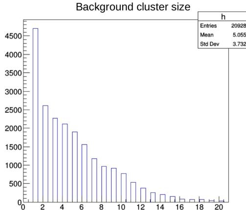
Figure 3: Cluster size of background hits after digitization. As can be seen in the plot, most of the background hits have a large cluster size.
