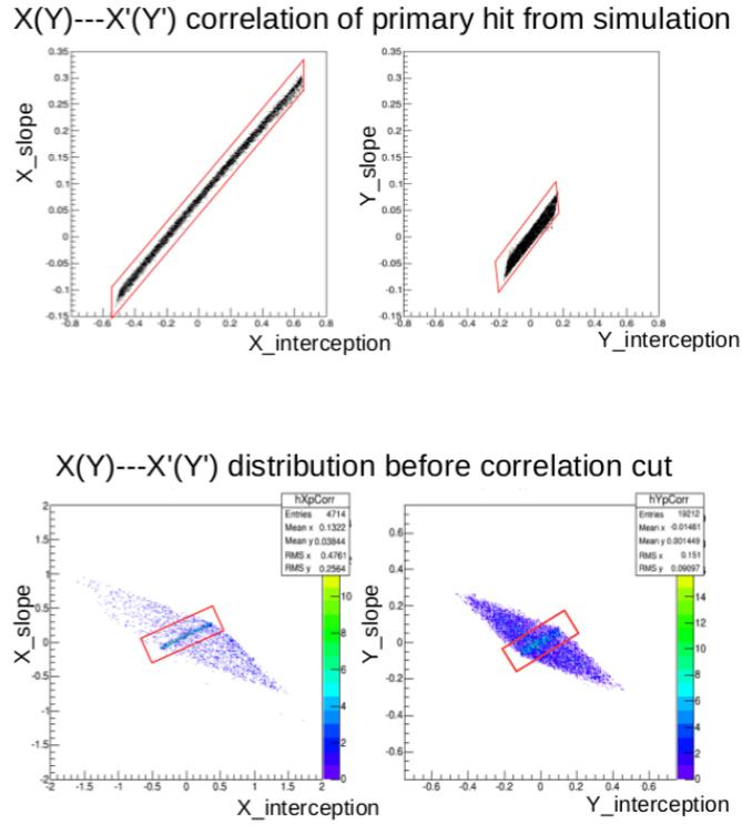
Figure 7: The top plot shows the correlation between slope and interception of a elastic track and the bottom plot shows the cut applied to reconstructed candidate tracks
