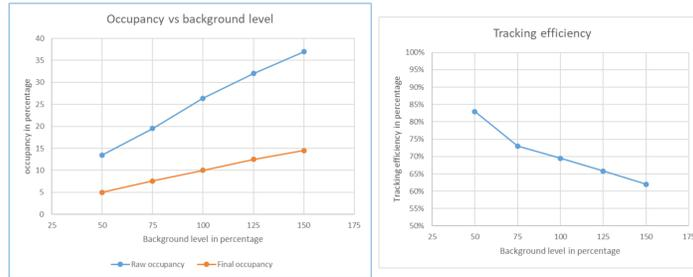
Figure 9: Occupancy level and tracking efficiency *vs.* background level. The GMn background estimated by simulation is denoted 100%. The raw occupancy includes all background hits within the readout window. The final occupancy excludes hits rejected at the hit reconstruction stage using timing information, and gives sense of background level that needs to be handled at the track reconstruction stage.
