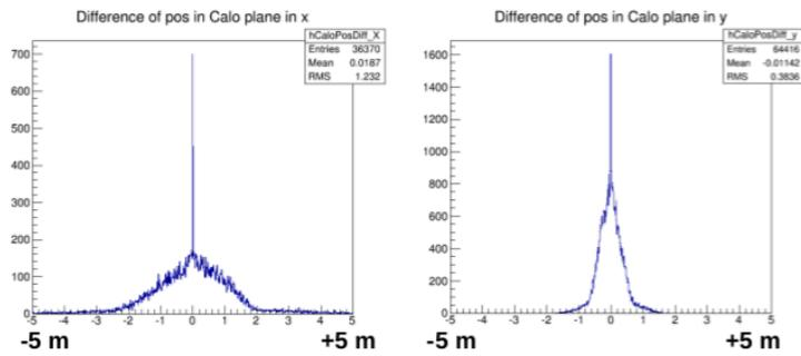
Figure 6: Calorimeter resolution and residual of primary hits' projected point in the calorimeter plane.
