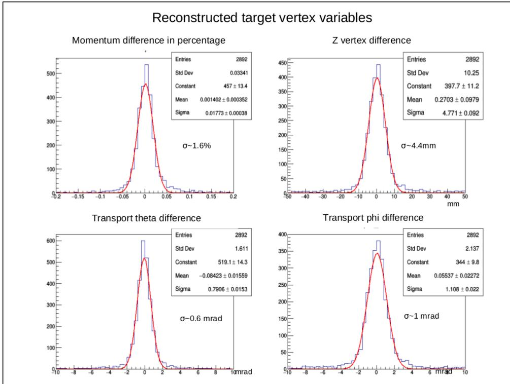
Figure 10: Accuracy of reconstructed target vertex variables at 100% estimated background level in the GMn experiment.
