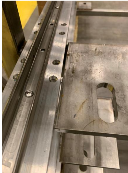
Top Track mount 2 nd from the back left side without fasteners Dec. 23 2020
