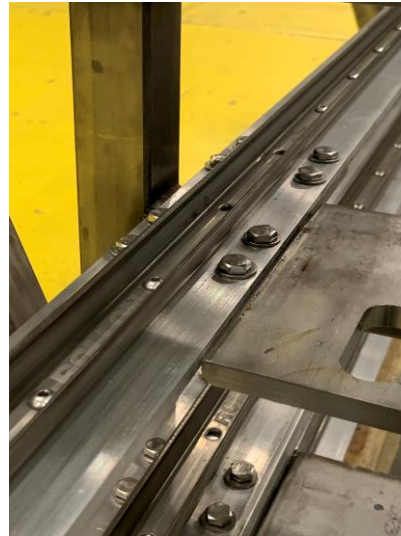
Top Track mount 2 nd from the back left side with fasteners Jan. 14 2021
