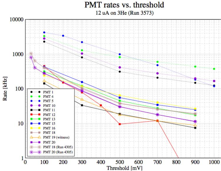
Figure 15: Background rates vs. discriminator threshold in the Cerenkov PMTs for  $12 \mu\text{A}$  on the  $^3\text{He}$  target during Transversity (BigBite at  $30^\circ$ ). Gains were matched so that the 1 p.e. signal had an amplitude of roughly 50 mV. PMTs 1–10 run from top to bottom nearest the beamline. PMTs 11–20 run from top to bottom on the far (RHRS) side of the BigBite stack.
