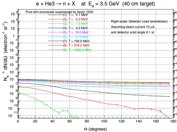
Figure 2: The neutron yield according to P. Degtyarenko’s calculation for the E02-013 target and 3.5 GeV beam (only the  $^3\text{He}$  and the glass cell were included in this calculation).
