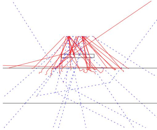
Figure 4: The GEANT display of the electron tracks (red lines) between the Ru-106 source, a scintillator counter (10x10 mm) and the PMT window.
