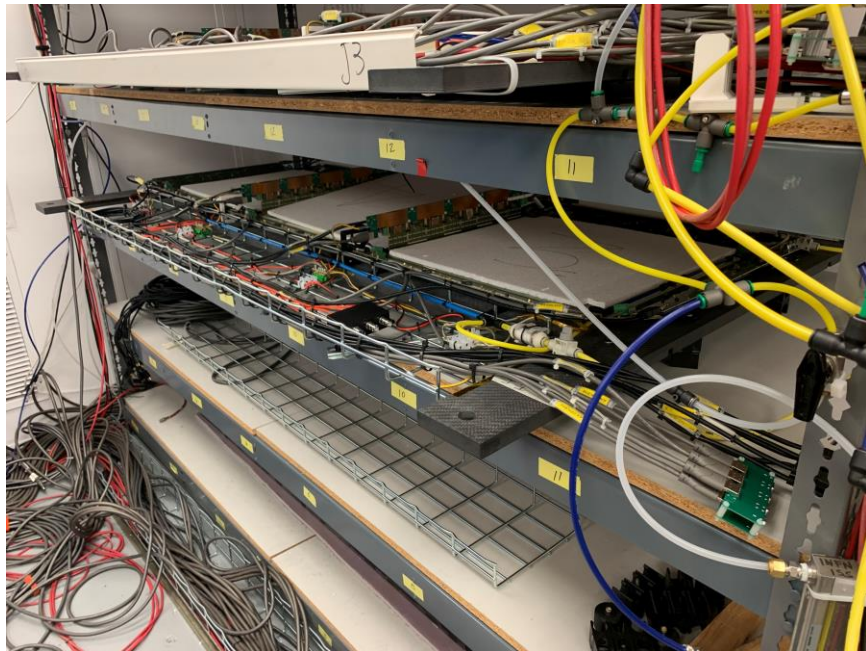
Top Left: Layer J1, DAQ side, with plastic cable tray Bottom Left: After J1 cable tray replacement, DAQ side Top Middle: Layer J1, door side, with plastic cable tray Right: After J1 cable tray replacement, door side
