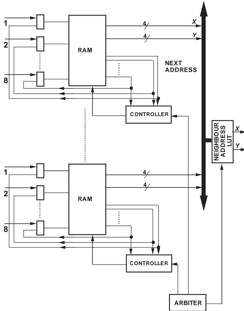
Figure 229: Schematic diagram of the Hit Address Memory block in the HFU.
