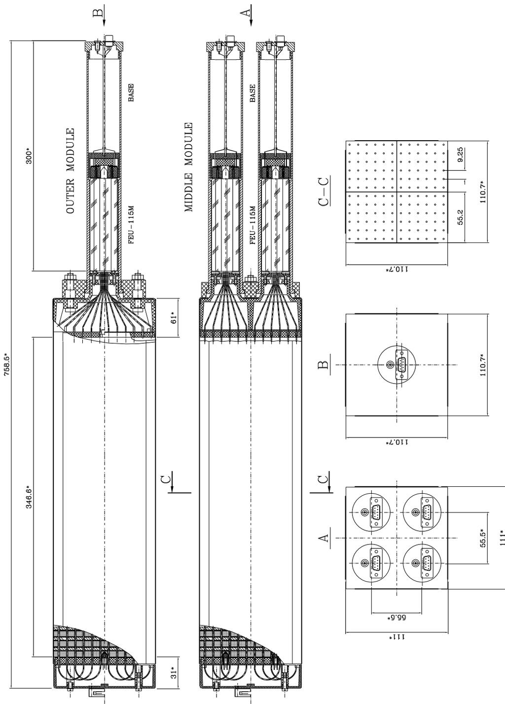
Figure 220: Drawings of the middle and outer modules.
