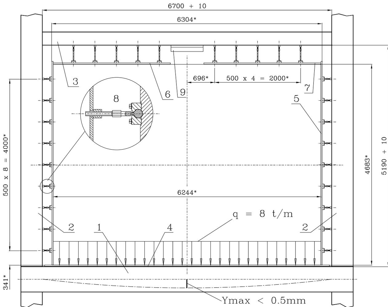
Figure 222: Conceptual view of the support structure installed on the middle platform.
