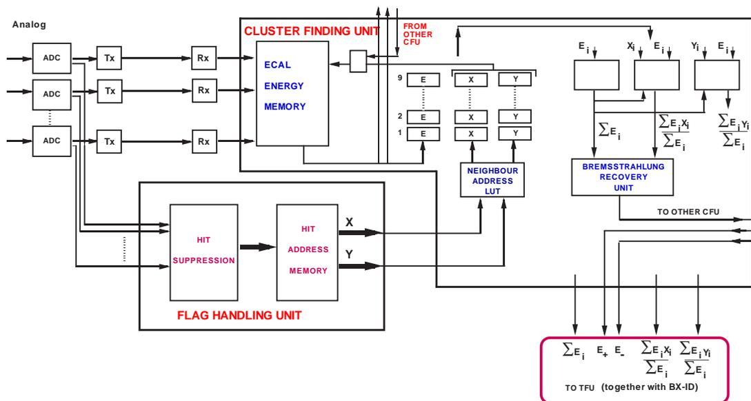
Figure 228: Block diagram of a possible ECAL pretrigger electronics scheme.
