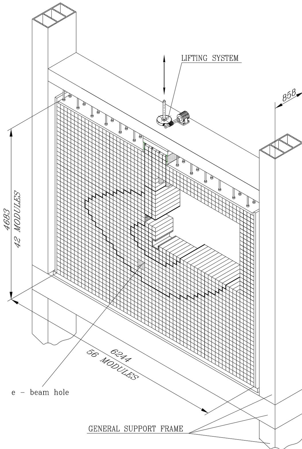
Figure 214: Isometric view of the calorimeter. Inner, middle and outer regions are separated by the bold plotted lines. The numbers are in mm.
