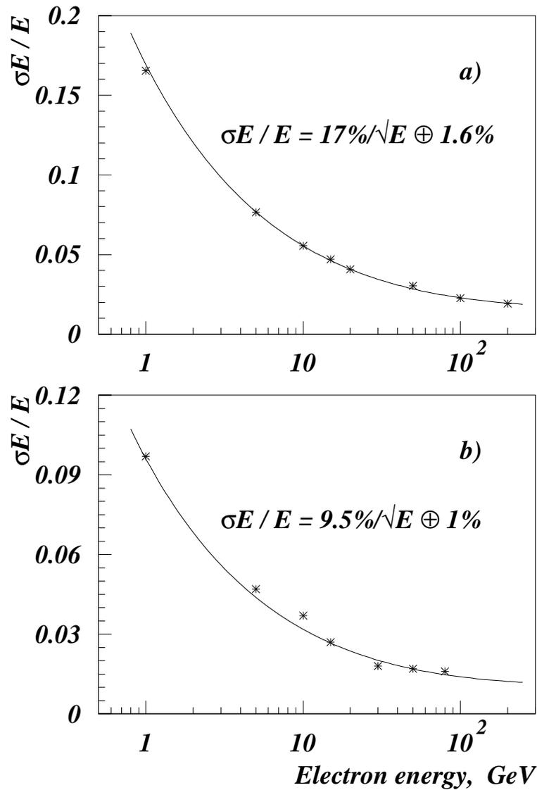
Figure 215: *Energy resolution of the inner (a) and middle/outer (b) ECAL modules.*
