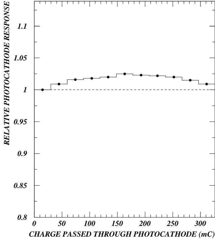
Figure 224: FEU-68 PM photocathode response as a function of the charge collected at the first dynode.
