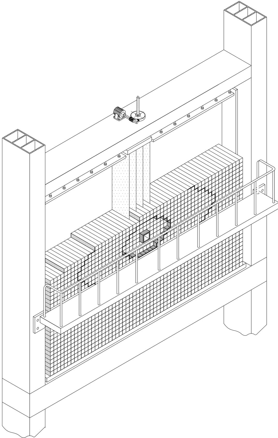
Figure 223: *Mounting of the ECAL modules into the support structure.*
