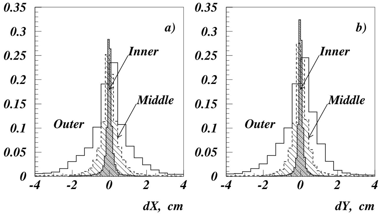
Figure 216: *Spatial resolution of ECAL modules in horizontal (a) and vertical (b) directions.*
