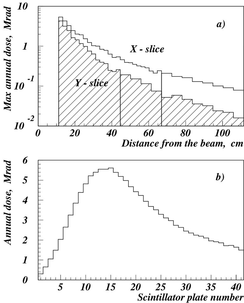
Figure 217: Annual radiation load of the calorimeter. (a) Dose accumulated at the shower-max position; boundaries between the inner and middle sections of the ECAL are shown by vertical lines. (b) Longitudinal annual dose distribution for the most loaded inner ECAL tower.
