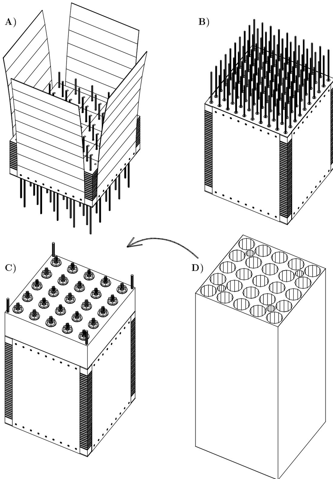
Figure 221: Assembly procedure of the inner module. (A)-stacking of the module; (B)-insertion of the WLS fibres; (C)-grouping the fibres into bundles; (D)-installation of the PM housing.
