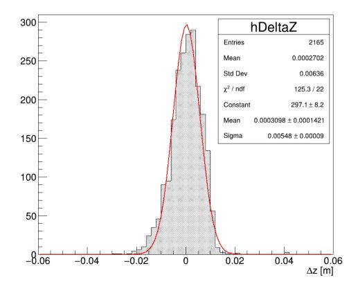
Determined relationship between fittled position of radius of first point of track in gas volume and Z. Difference between expected and actual z gave 6mm sigma width resolution number for z-resolution estimate.
