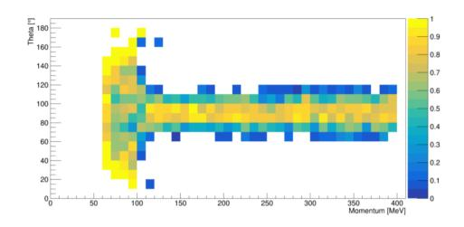
Conical design – tracks which do not hit either HV plane or readout Tracks randomnly generated across theta 0-180deg, all phi, momentum 60-400MeV/c
