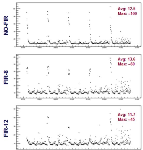
Measured RMS pedestal noise levels for MPD APV electronics. This test was done for a set of 5 APV cards. Horizontal axis shows the strip number where the vertical axis is pedestal noise level in units of ADC channels. One ADC channel is equivalent to approximately 160 e-.
