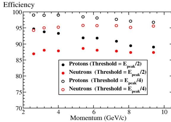
Figure 1.8: Detection efficiency in a  $3 \times 3$  cluster in the hadron calorimeter for protons and neutrons for GMn [2] kinematics. Results are from GEANT4 simulations.
