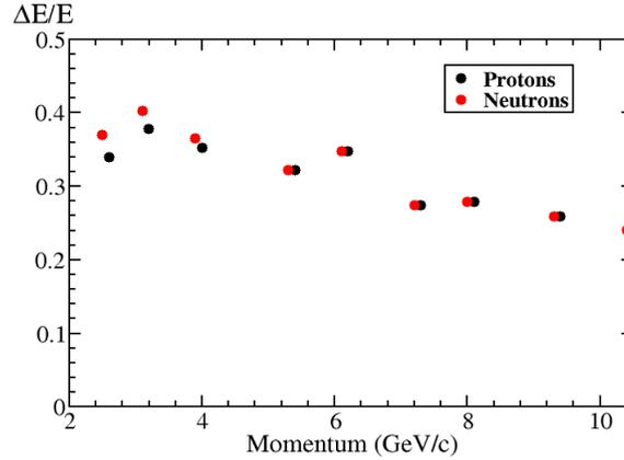
Figure 1.7: Resolution of the deposited energy in a  $3 \times 3$  cluster in the hadron calorimeter for protons and neutrons for GMn [2] kinematics. Results are from GEANT4 simulations.
