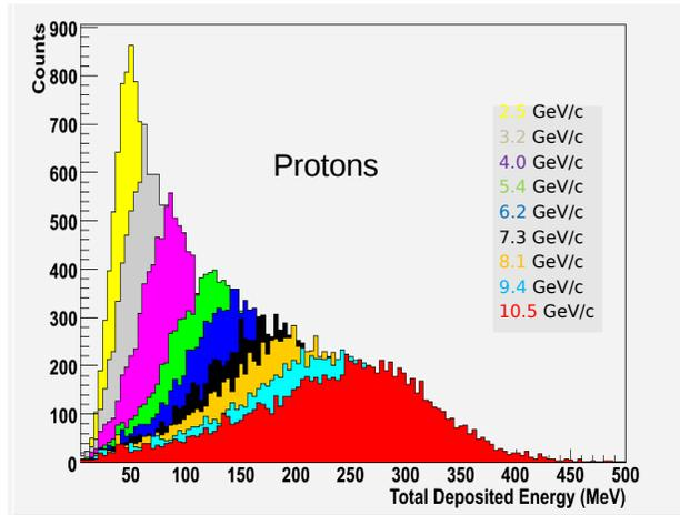
Figure 1.5: Energy deposited in a  $3 \times 3$  cluster in the hadron calorimeter corresponding to protons for GMn [2] kinematics. Results are from GEANT4 simulations.
