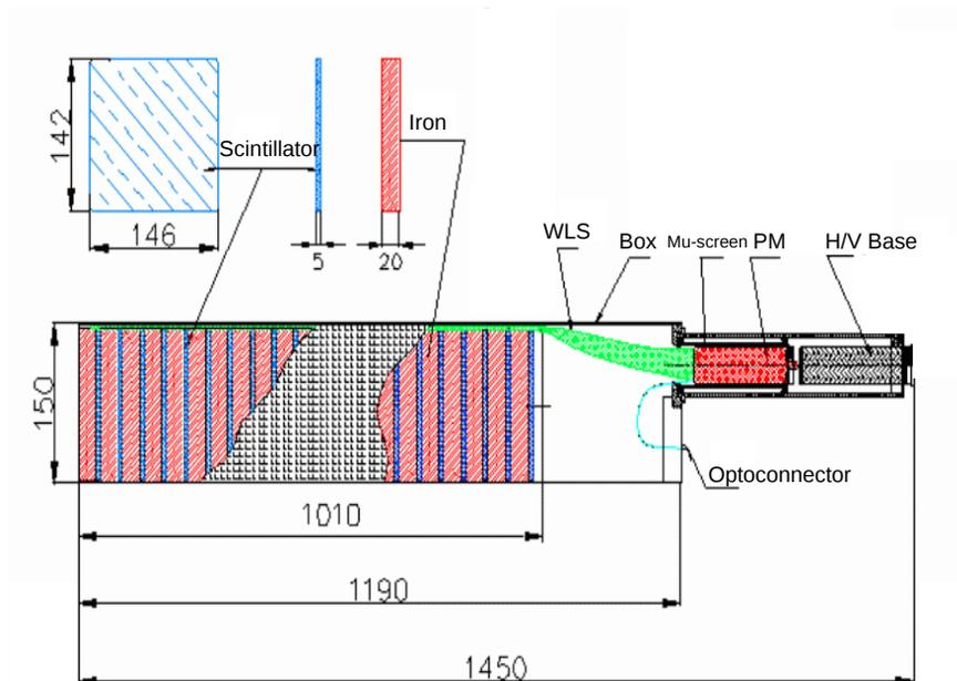
Figure 1.2: One module of COMPASS *HCAL* hadron calorimeter [5]. All dimensions are in mm.
