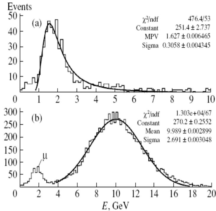
Figure 1.3: Spectra of the energy deposited in a *HCALI* module by (a) muons and (b) pions at a beam energy of 10 GeV [5].
