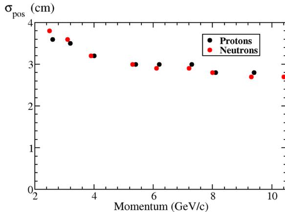
Figure 1.9: Position resolution for a  $3 \times 3$  cluster in the hadron calorimeter for protons and neutrons for GMn [2] kinematics. Results are from GEANT4 simulations.
