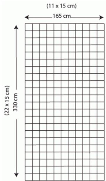
Figure 1.1: HCAL for Super-Bigbite with 242 modules of iron/scintillator plates arranged in a matrix  $11 \times 22$ .
