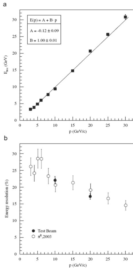
Figure 1.4: COMPASS *HCAL1* (a) energy reconstruction and (b) energy resolution as a function of momentum for identified hadrons (the full symbols denote test beam results) [6].
