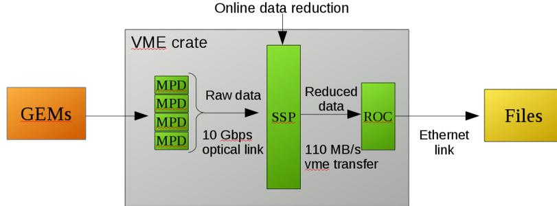
Figure 1: Data flow chart of the current SSP based system. The MPD digitizes signals from APV cards on the GEMs and send it to an SSP. Groups of 4 MPDs share a 10 Gbps optical link which fed into 1 of 8 optical ports on each SSP. Real time data reduction is performed by the SSP which then sends reduced data through VME backplane which has an average transfer rate of 110 MB/s to the crate’s readout controller (ROC).
