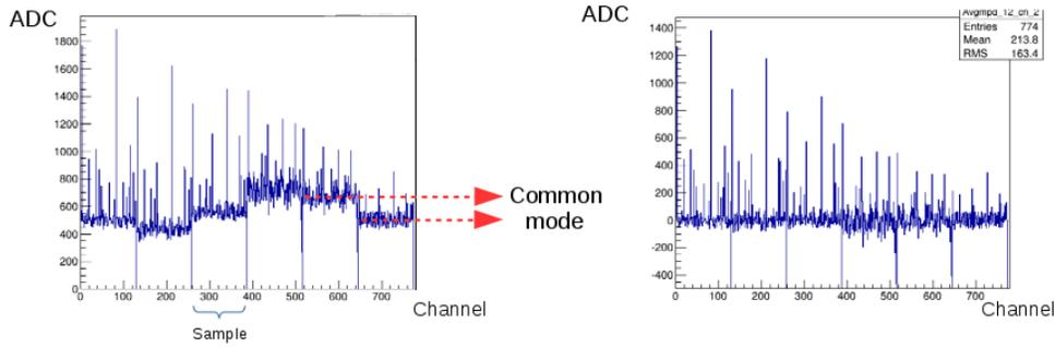
Figure 2: Plot on the left shows how the ADC baseline of channels in one APV fluctuates from sample to sample. These shifted baselines need to be identified and offset before applying a threshold cut for zero suppression. Channels that legitimately fire within a group need to be identified and excluded from the baseline identification. Plot on the right is after common mode correction.
