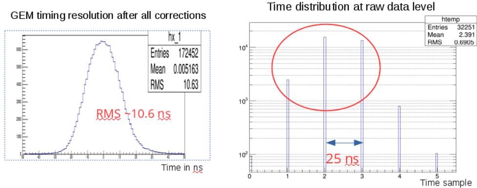
Figure 4: The final timing correlation of good hits with trigger has RMS around 10 ns after corrections (left plot). In the raw channel data before any correction, the timing of a good hit is localized to within 3–4 25 ns time samples. Channels with timing out of this range can be identified as background and suppressed.
