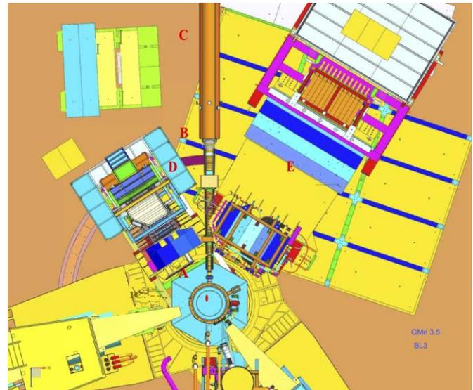
Fig. 1. Illustration to the general layout of the GMn beam line and other equipment in the vicinity. The capital letters (A, B, C, D, E) indicate the regions of interest for the calculations of residual radioactivity during and after the run.
