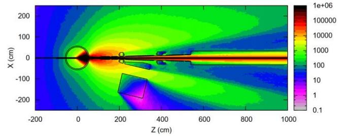
Fig. 4. Prompt total dose equivalent rates in the horizontal layer 30 cm thick during the run at 8.8 GeV beam energy and 30  $\mu$ A beam current.
