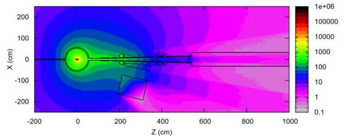
Fig. 7. Prompt neutron dose equivalent rates in the horizontal layer 30 cm thick during the run at 4.4 GeV beam energy and 22  $\mu$ A beam current.
