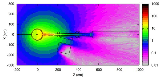
Fig. 10. Total dose equivalent rates in the horizontal layer 30 cm thick, 24 hours after the end of 64-hour continuous irradiation during the run at 8.8 GeV beam energy and 30  $\mu$ A beam current.
