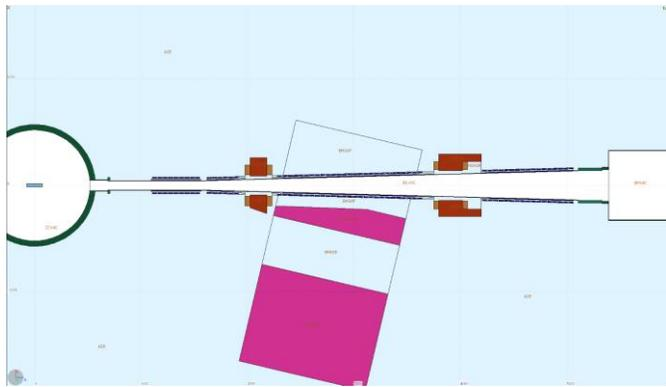
Fig. 3. Horizontal plane cut view of the FLUKA model for the GMn beam line. Cylindrical volume of the Interaction Chamber contains the target inside. The beam exit line is modeled as a pipe with flanges, then conical volume with a set of iron magnetic shielding rings around it, exiting into a large-diameter exit pipe leading to beam dump. The beam control quadrupole magnets, as well as the movable big magnet surround the beam line.
