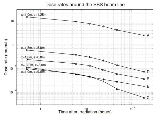
Fig. 11. Evaluated dose rates in the five locations around the beam line (A, B, C, D, E as referenced in Fig. 1), function of time after irradiation, from 30 minutes to 1 week. The locations are within  $\pm$  15 cm of the horizontal plane, in the vicinity of the (x,z) coordinates indicated next to each series.
