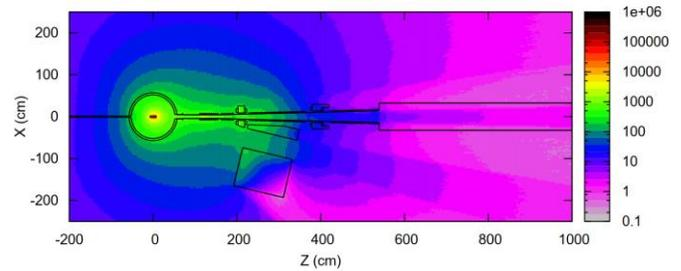
Fig. 5. Prompt neutron dose equivalent rates in the horizontal layer 30 cm thick during the run at 8.8 GeV beam energy and 30  $\mu$ A beam current.
