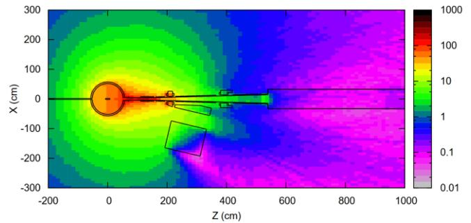
Fig. 9. Total dose equivalent rates in the horizontal layer 30 cm thick, 30 min after the end of 64-hour continuous irradiation during the run at 8.8 GeV beam energy and 30  $\mu$ A beam current.
