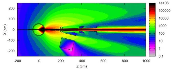
Fig. 6. Prompt total dose equivalent rates in the horizontal layer 30 cm thick during the run at 4.4 GeV beam energy and 22  $\mu$ A beam current.
