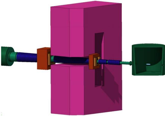
Fig. 2. 3D view of the FLUKA model for the GMn beam line. Cylindrical volume of the Interaction Chamber is cut out to show the location of the target inside. The beam exit line is modeled as a pipe with flanges, then conical volume with a set of iron magnetic shielding rings around it, exiting into a large-diameter exit pipe leading to beam dump. The beam displacement control quadrupole magnets, as well as the movable big experimental magnet surround the beam line.
