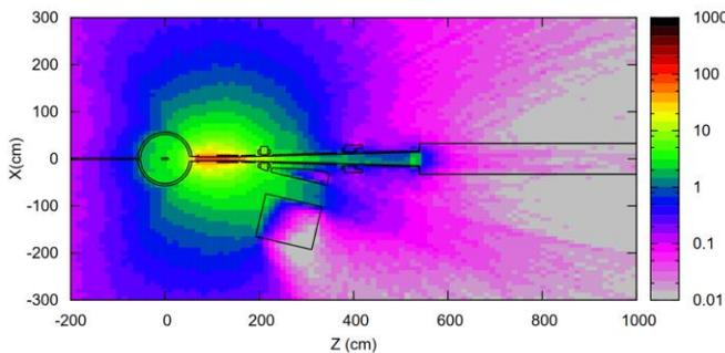
Fig. 8. Dose equivalent rates in the horizontal layer 30 cm thick, 64 hours after the end of 724-hour continuous irradiation during the run at 4.4 GeV beam energy and 22  $\mu$ A average beam current.
