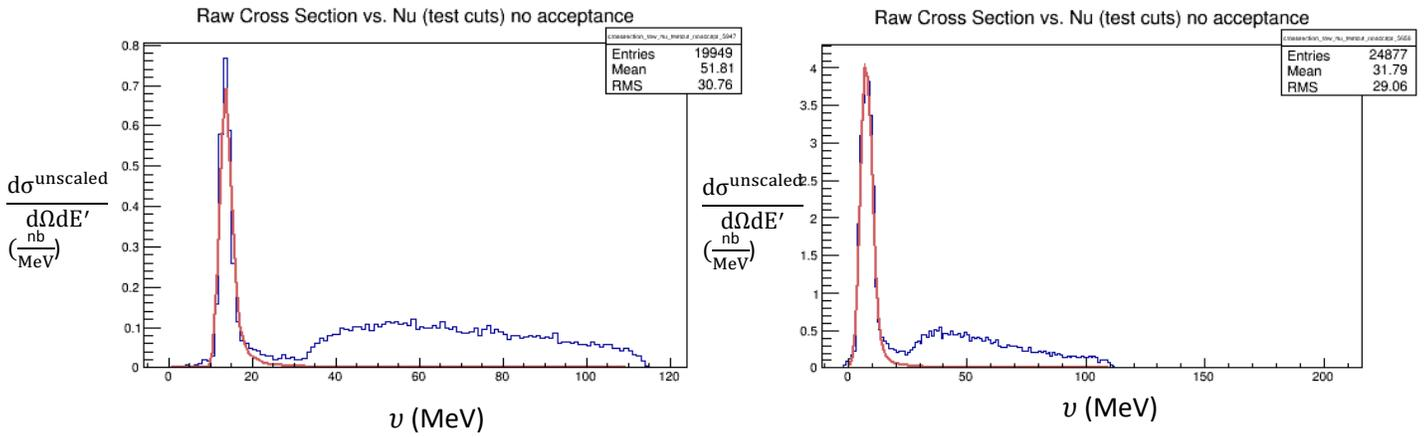
Figure 1: Unscaled cross sections for empty runs with elastic peak fits. Longitudinal setting on run 5650 (left) and transverse setting on run 5947 (right)
