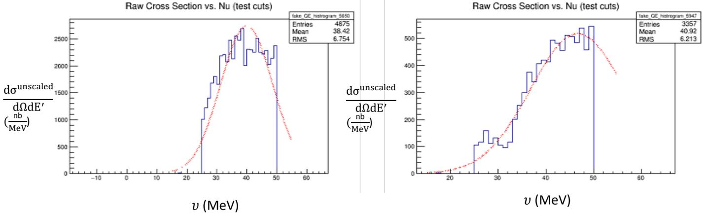
Figure 2: Cross sections for the empty runs with only quasielastic data, with fake data at 15 MeV to force the Gaussian fit to go to zero. Longitudinal setting on run 5650 (left) and transverse setting on run 5947 (right)
