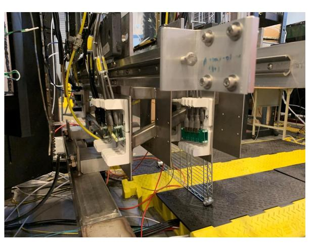
• All the HDMI cables on both J0 and J2 reach wire holders, as designed.
