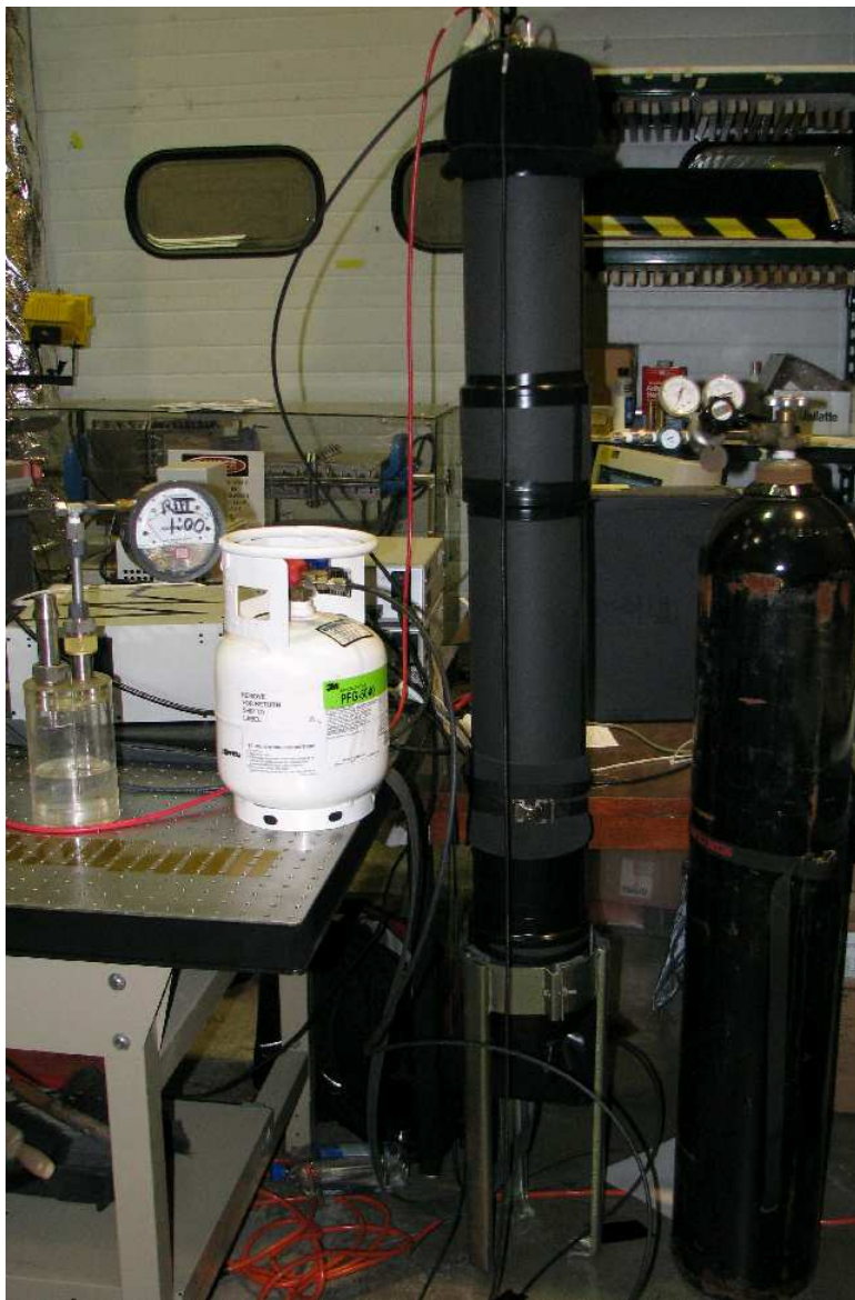
Figure 6: Another view of the experimental setup. In the center is the dark tube; the PMT is located at the top of the tube. The red wire is the high voltage for the PMT. The black hoses coming from the top and bottom of the tube, the gas tanks, and the bubbler (far left, on table) are used for pumping gas into the tube.
