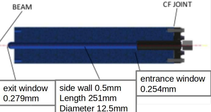
Since we have a very "thin" target comparing to the aluminum endcaps, the endcap contamination must be carefully removed in analysis by comparing to the empty cell.
