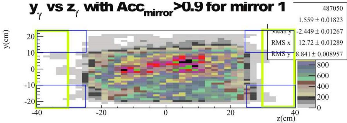
**Figure 18. Simulation used to Find 'Extreme' Photons.** This image shows where photons will strike a mirror and how many will strike that position. The four corners of the mirror were examined to find the photons that would come closest to not striking the PMT array.
