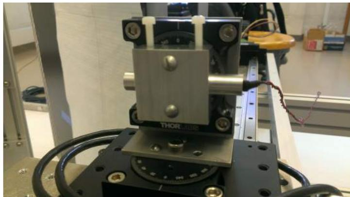
**Figure 3. Laser Mount.** This mount allows for the laser angle to be adjusted horizontally and/or vertically.
