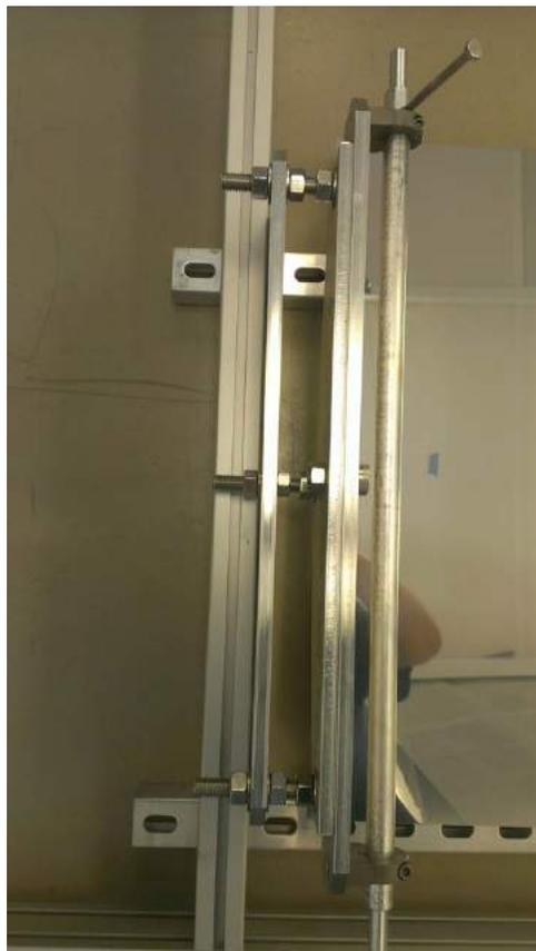
**Figure 2. Radius of Curvature Adjustment Methods.** The radius of curvature of the mirror can be adjusted by moving the positions of the nuts or by twisting the lever seen at the top of the figure.
