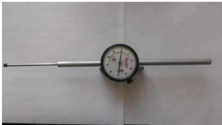
**Figure 12. Dial Drop Indicator.** This dial drop indicator was used to measure the depth of the mirror due to the curvature. This allowed the radius of curvature to then be calculated.
