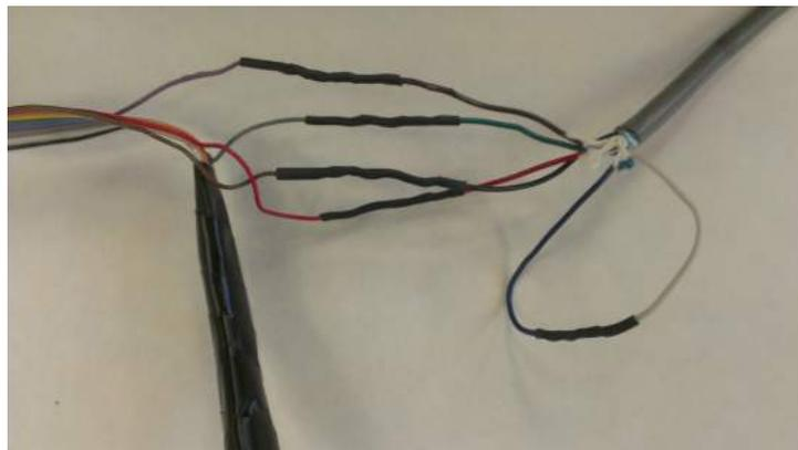
**Figure 5. Motor Controller Wiring.** The rainbow cable on the left connects to the motor controller and the gray cable on the right connects to the linear rail system. The wires, listed from controller to linear rail system, are connected as follows: purple-to-brown, gray-to-green, brown-to-black and red-to-red. Also the blue and white wires both originating from the gray cable connecting to the linear rail system were connected to one another in a loop.
