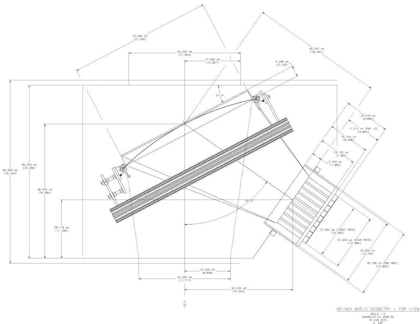
**Figure 17. GRINCH Detector Geometry.** This image shows the detector geometry which was replicated for testing. This image can also be found on the JLab GRINCH wiki page under design.
