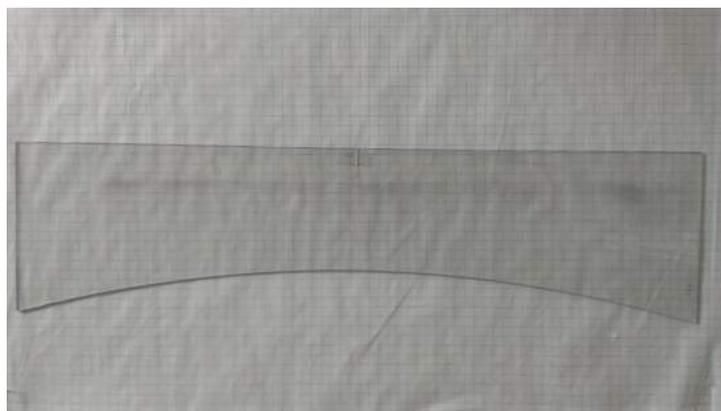
**Figure 6. Plastic Guide.** This guide is cut to a radius of curvature of 130 cm. By placing it on the back of the mirrors while aligning them a more accurate radius can be achieved.
