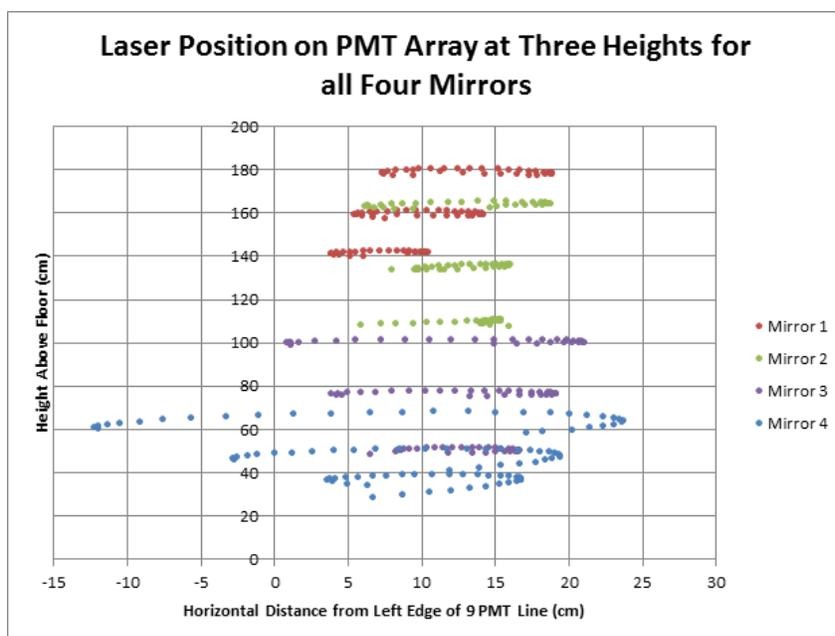
**Figure 23. Full Mapping of Laser Paths on PMT Array.** This graph shows the path a laser fired at zero degrees onto the mirrors takes on the PMT array at three levels per mirror. Note in this image zero is the left edge of the 9 PMT line not the central line of the PMT array.
