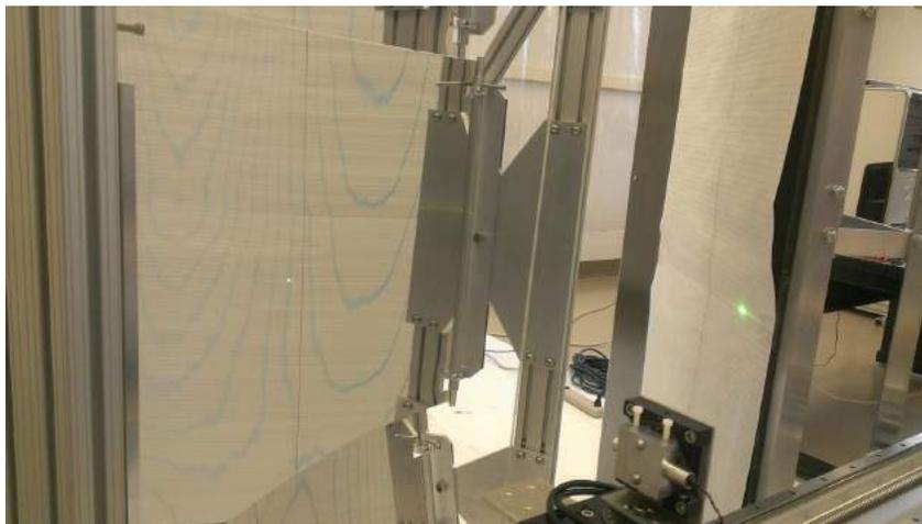
**Figure 16. Laser Reflecting onto PMT Array.** The laser can be seen reflecting off of the mirrors and striking the simulated PMT array on the right side of the image.
