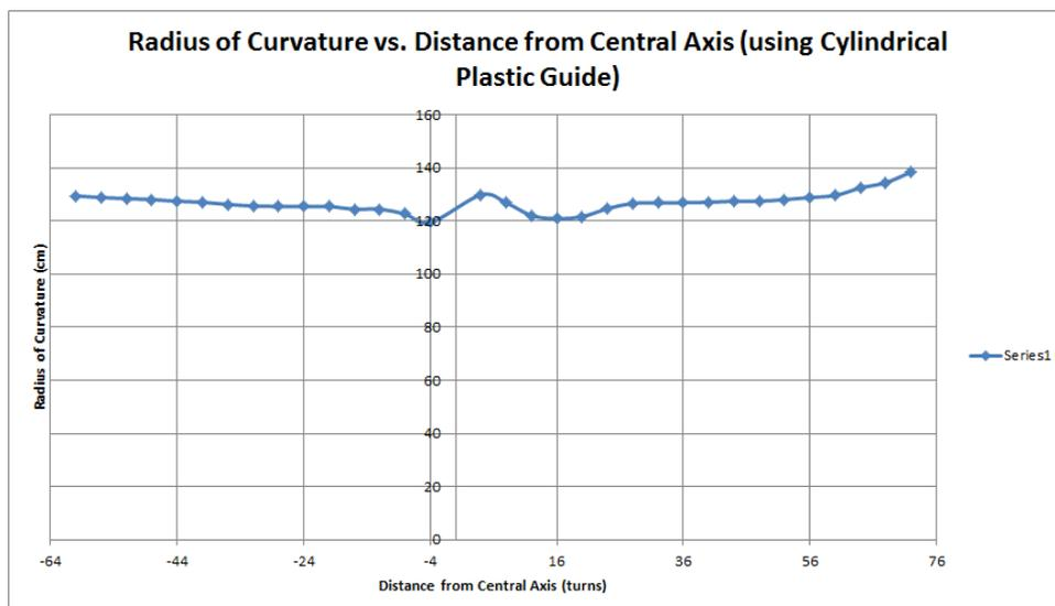
**Figure 7. Radius of Curvature Test.** This test was performed while the plastic guide was secured to the back of the mirror on the central horizontal line.
