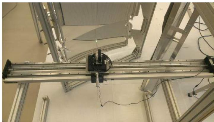
**Figure 4. Linear Rail System.** This rail allows for the laser to be moved across the face of the mirror.
