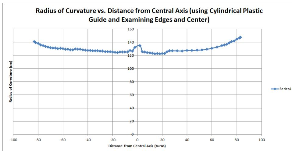
**Figure 8. Radius of Curvature Test New Alignment.** This test was performed while the plastic guide was secured to the back of the mirror on the central horizontal line. The data were taken after the mirror had been aligned separately from the alignment seen in Figure 7.
