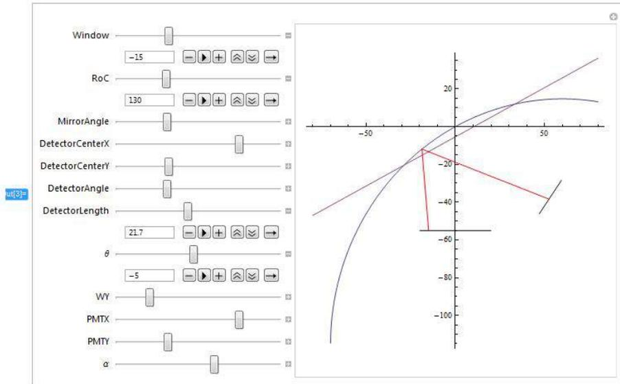
**Figure 21. Mathematica Simulation of Mirror System.** The horizontal black line represents the entrance window and the angled black line represents the surface of the PMT array. The blue circle represents the mirror surface with the purple line showing the approximate size of that surface. Lastly the red line represents the ray formed by a photon entering the detector and reflecting off of the mirror.
