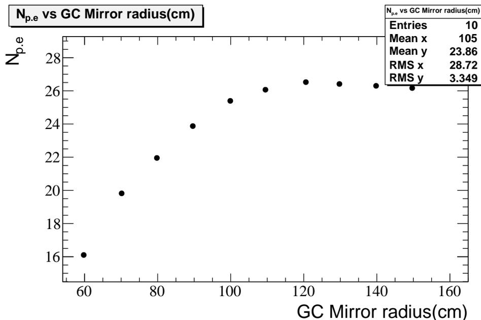
**Figure 9. Radius of Curvature Efficiency Simulation.** This simulation provided by Huan shows the photon collection efficiencies of various radii of curvature. Around 130 cm there is considerable tolerance in radius variations before photons are lost.
