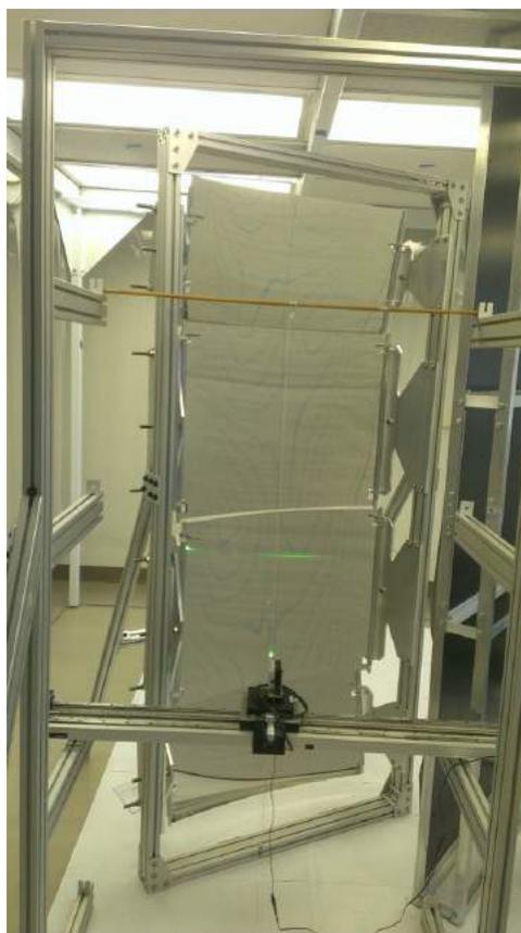
**Figure 14. Mirror Frame.** A frontal view of the mirror frame holding the four prototype mirrors. In the foreground the linear rail system with the laser can be seen on an independent frame.
