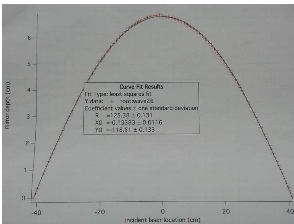
**Figure 13. Dial Drop Indicator Measured Radius of Curvature.** This fit was done in Igor Pro. The red crosses represent the experimental data and the black line the fit of this data.
