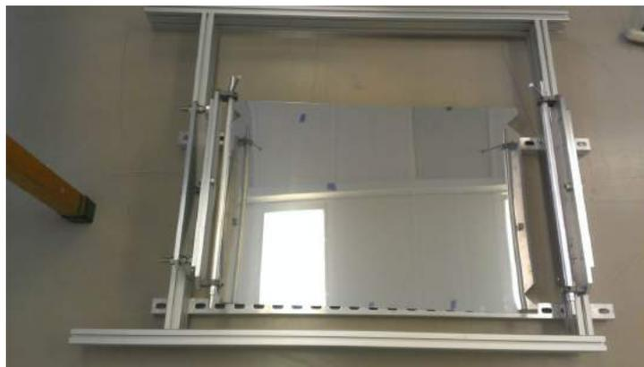
**Figure 1. Mirror Frame Prototype.** Note: Mirror is held by the two vertical rods during testing.
