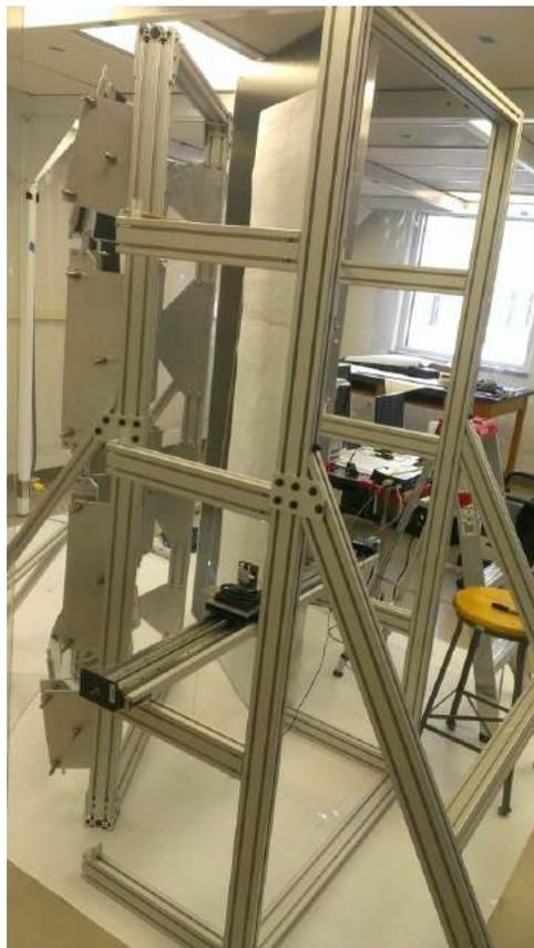
**Figure 15. Laser Frame.** In the foreground the frame holding the laser and linear rail can be seen. Each of the four levels on this frame can be moved up or down. A side view of the mirror frame can be seen on the left. In the central background the black rectangle with paper attached to it represents the PMT array.
