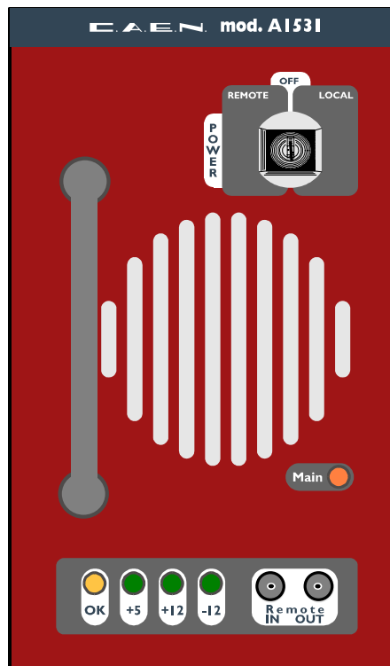
Fig. 3.3 – Front panel of the Primary Power Supply (Mod. A1531)
