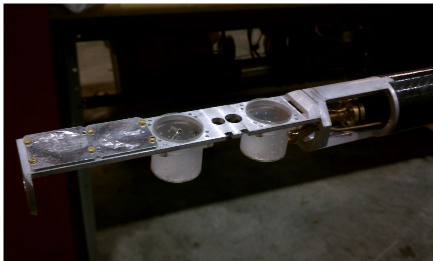
Figure 4: The ladder of the new target inserts, showing both target cups and microwave horn.
