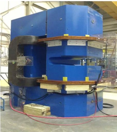
Figure 1a SBS Magnet when being tested at 200A
