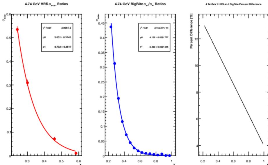
**Figure:** Left plot has the LHR5  $e^+e^-$  ratio fitted with an exponential function, the center plot has the BB  $e^+e^-$  measured using different polarities and fitted to an exponential function. The right most plots shows the percent difference between the LHR5 and BB fits. There is a large disagreement at low  $x$  with agreement improving as  $x$  increases.
