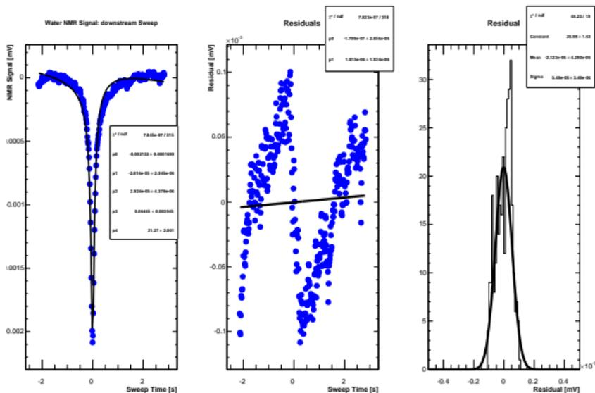
Figure: Left Plot shows the water NMR signal and fit. Center plot shows residual between data and fit with linear fit. The right plot shows residual histogram fitted with a Gaussian fit.
