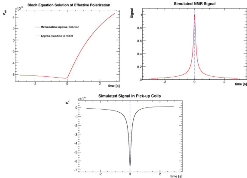
**Figure:** Top left plot shows the solution to the effective polarization. The top right plot shows the signal shape of the NMR signal. The bottom plot shows the simulated shape in the RF coils.
