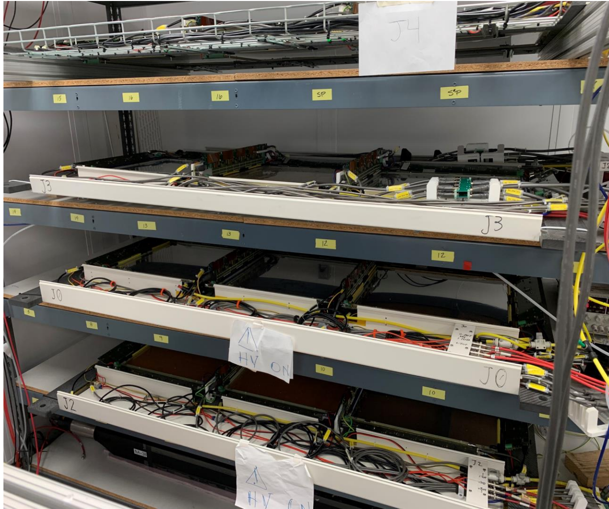
From top to bottom DAQ side: J4 (metal), J3 (plastic), J0 (plastic), J2 (plastic). Priority is J0 and J2, since best chambers
