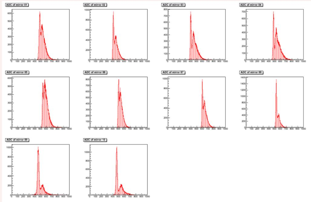
Figure 2: Plots of not calibrated 10 nearside PMTs ADC spectra.
