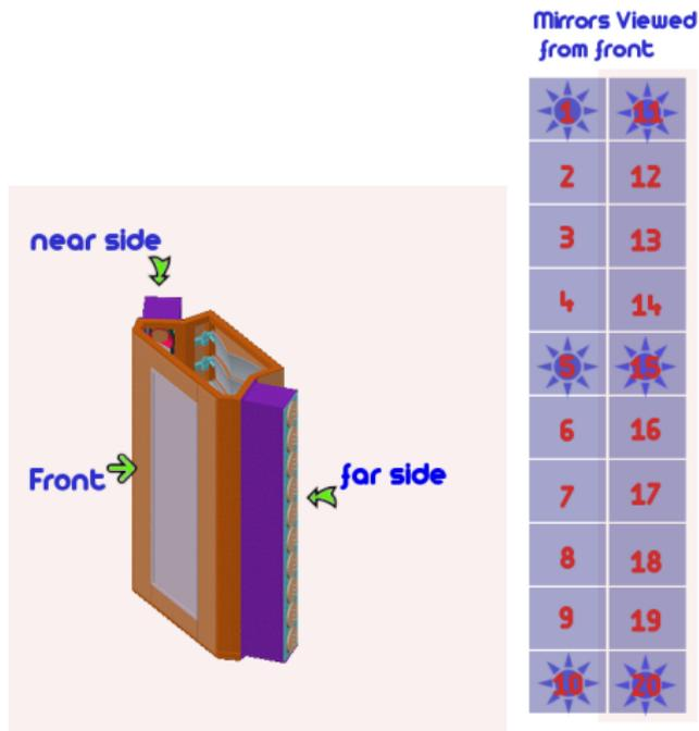
Figure 1: CAD rendering of the Big Bite Cerenkov and layout of the mirrors corresponding to the PMTs, the blue suns mark the location of the LEDs during the LED run.
