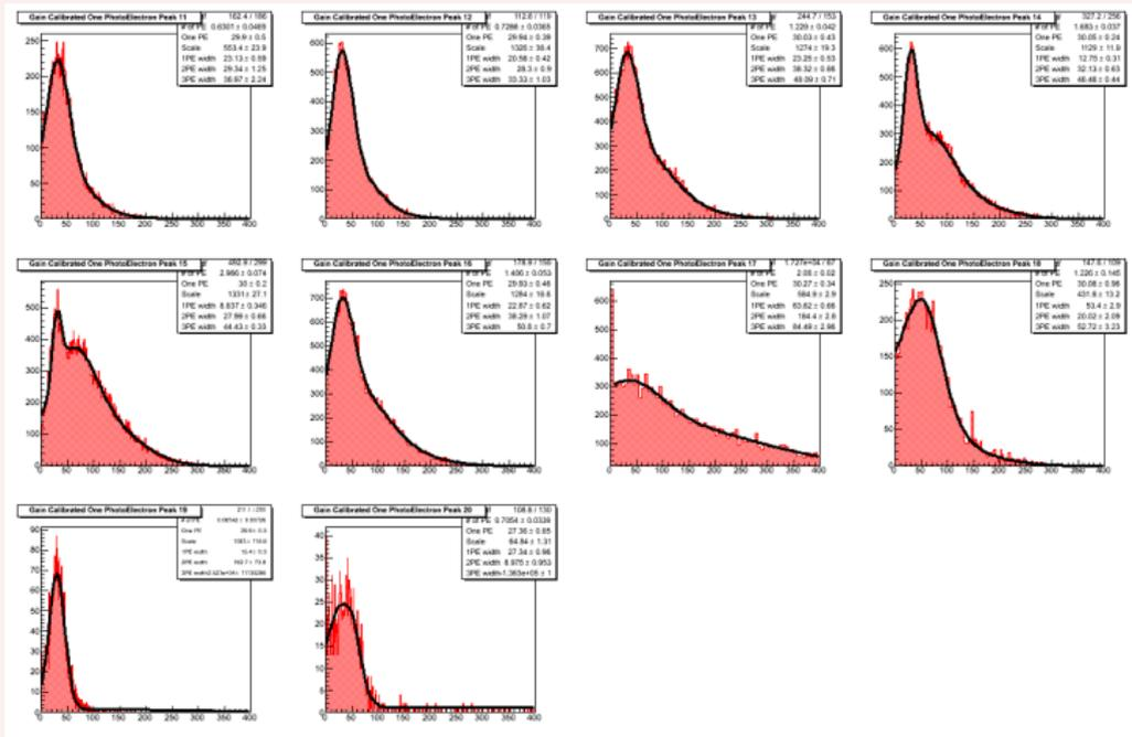
Figure 5: Plots of fitted 10 farside PMTs ADC spectra.
