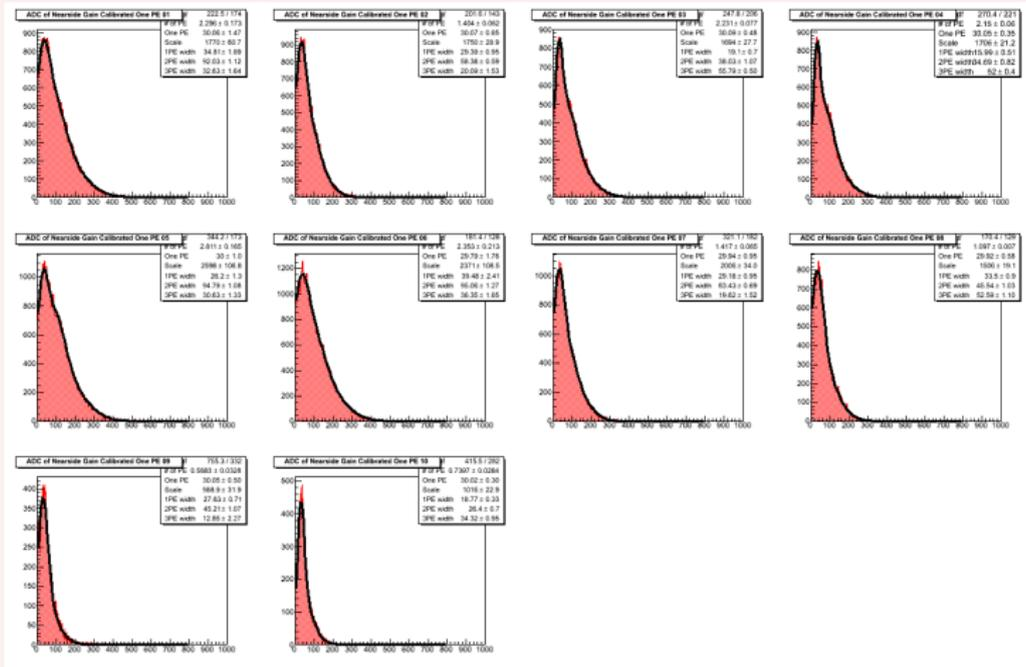
Figure 3: Plots of fitted 10 nearside PMTs ADC spectra.
