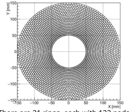
There are 21 rings, each with 122 pads, (2 562 total pads per readout plane).
