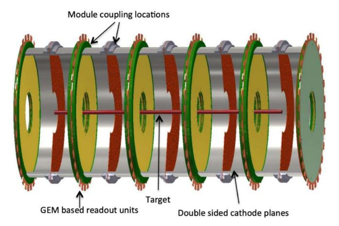
The mTPC will consist of 10 separate TPC volumes. The entire detector will be 55 cm long. Inner radius of 5 cm and an outer radius of 15 cm.
