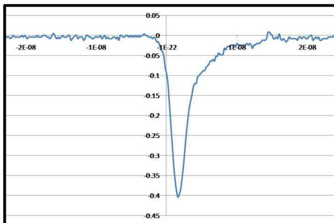
**Figure 3.** The scope view of an example neutron spike shows that the pulses have width between 4-5 ns with a sharp leading edge rise time and a slight tail at the fall time.
