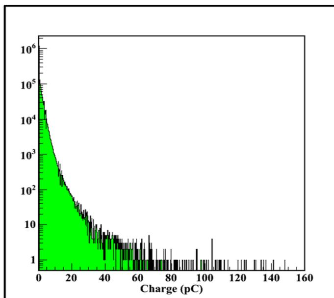
**Figure 5.** The pedestal subtracted ADC charge distribution of 20,000,000 triggers from Hamamatsu R7525-HA PMT. Distribution includes  $\times 10$  amplification, and every bin corresponds to 0.1 pC charge.
