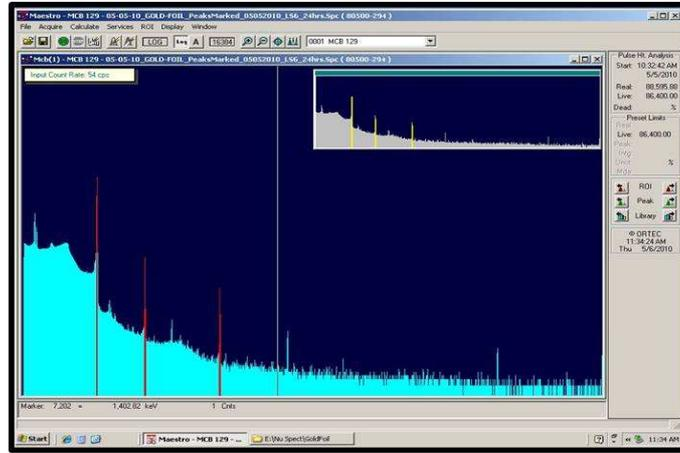
**Figure 2.** The screen output of the emitted gamma spectrum from gold foil, during 24 hours of HPGe detector measurements. The 411 keV photons were counted to determine the neutron flux on foil.
