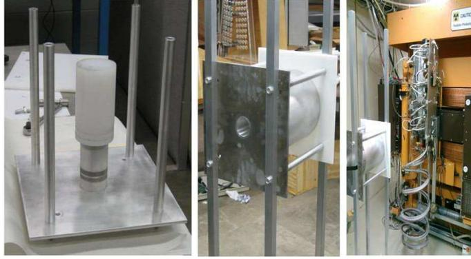
**Figure 1.** (LEFT) The polyethylene cavity at the center of the thermalizer. (MIDDLE) Back view of the finished thermalizer, with the well to insert PMT into the cavity. (RIGHT) The thermalizer is positioned 1 m away from the target of the cyclotron machine.
