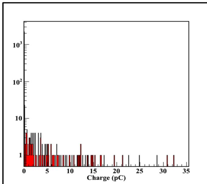
**Figure 4.** The pedestal subtracted ADC charge distribution of 10,000,000 triggers from Hamamatsu R7600U-200-M4 PMT. Distribution includes  $\times 10$  amplification, and every bin corresponds to 0.1 pC charge.
