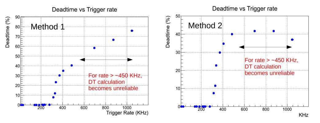
From B. Moffit's excel sheet, we get max rate = 468KHz for Integration window = 70(280ns)
