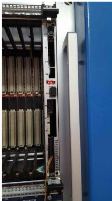
**Figure 4. TI taking Data.** This image shows the TI while it is taking data. Three lights are lit indicating data is being seen and recorded.
