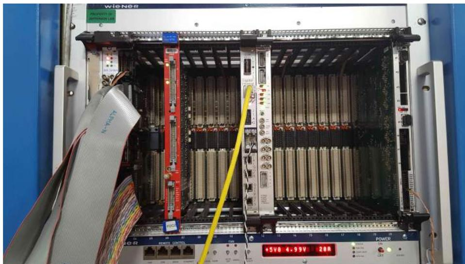
**Figure 7. VXS Crate Configuration.** This figure shows how the VXS crate looks when properly configured. NOTE: The red unit is an ADC and it is not utilized in the setup described here.
