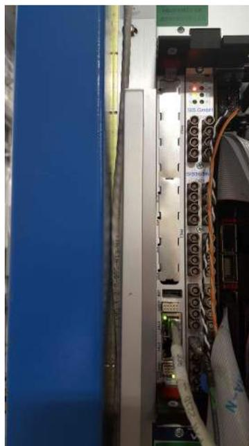
**Figure 8. Close Up of VXS CPU.** This figure shows a close up of the VXS CPU (left-most module) and its connections.
