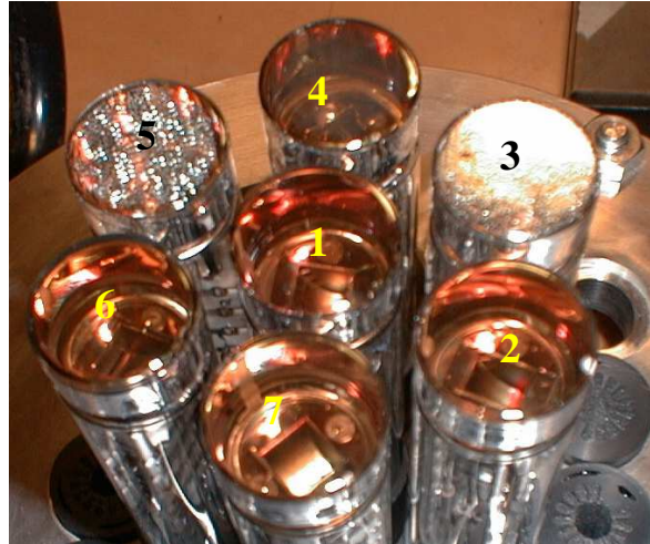
Figure 7. Appearance of seven PMTs, as the beginning of the corrosion test. One can see four “clear” PMTs on the bottom, two “frosty” on each side, and one “milky” at the top right-hand side.
