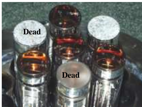
Figure 10. The same PMTs as in Fig. 7, after the third and fourth immersion in hot water for 174 days (equivalent to 82 months at 28°C); it is the second and third immersion for PMT #3’ and 7’. There are more scratches on four of the “milky” PMTs and the “frosty” PMT appears much more “frosty” when dry.
