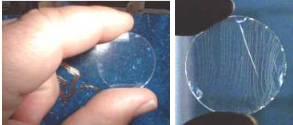
Figure 15. (a) B53 glass window coupon after the first immersion in water, and (b) after the third immersion.
