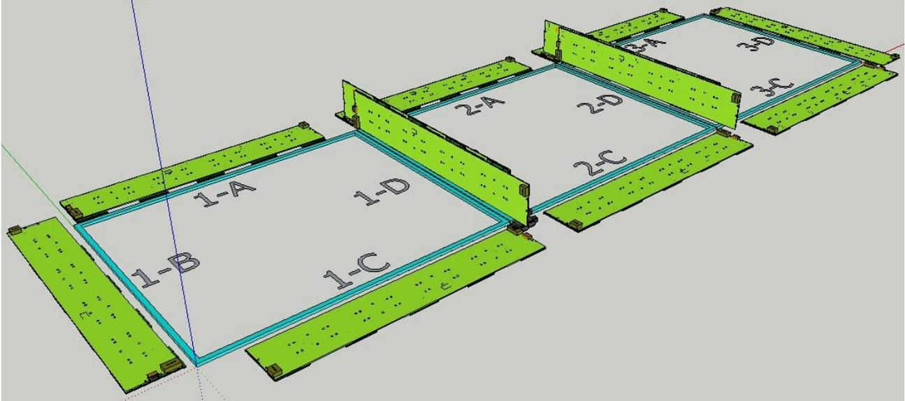
**Figure 2: Electronics layout in a chamber, on plane all around the 3 modules and vertical between modules; the green PCB are the backplanes.**
