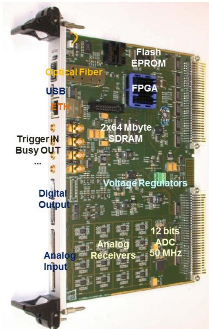
Figure 3: VME custom module MPD (Multi-Purpose Digitizer, version 3) for the control and readout of the front-end cards.
