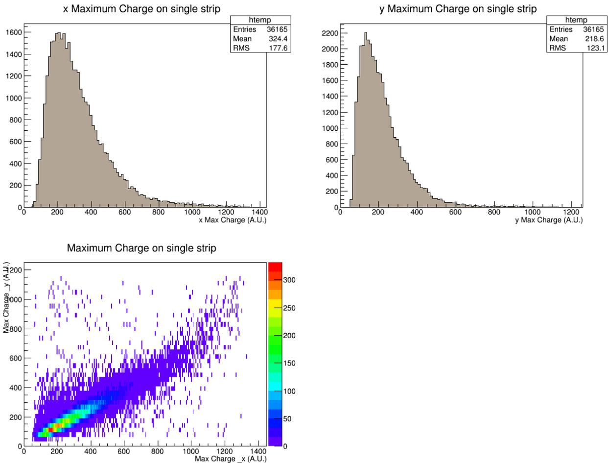
**Figure 7: ADC distribution (x and y strips) for the strip with maximum charge, obtained with a HV of 4100 V (gain of approx. 4800).**
