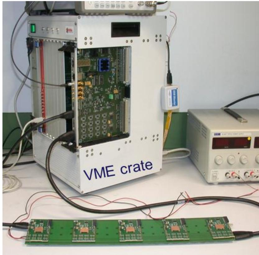
**Figure 1: MPD-INFN system components: the front end card (FEC), the backplane that can host up to 5 cards, the VME controller in VME64x standard; cards and MPDs communicate by HDMI cables.**
