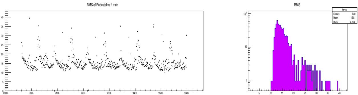
Figure 5: RMS pedestals for 5 cards connected to the y strips (40 cm long strips) in beam test environment (DESY/2014); average noise level is 15.5 ADC units; the analogue HDMI cable is 6 meter long.
